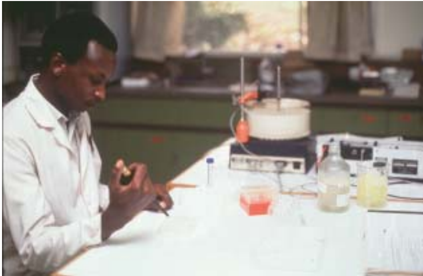
A research officer carrying out a chequer-board titration for human IFN-ELISA at the Kenya Medical Research Institute, Nairobi.
