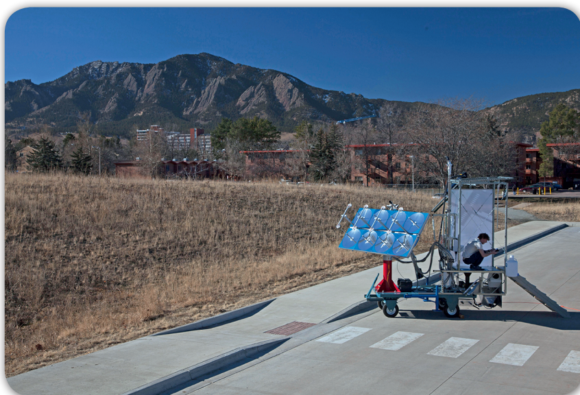
The Sol-Char toilet developed at the University of Colorado, Boulder, USA
