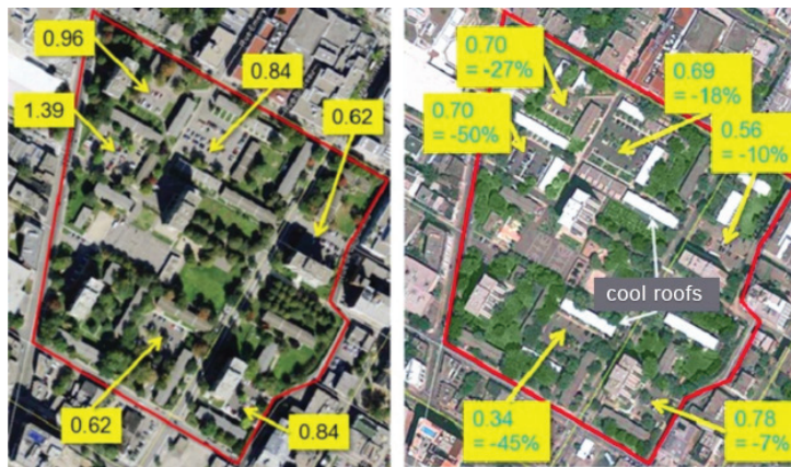
Note: Numbers in blue show a value decrease of normalized temperature implying a reduction of the UHI effect. Source: Environment Canada, Ottawa, Ontario, Canada.
